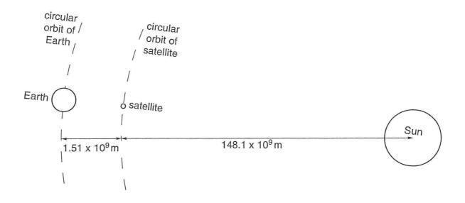
The speed of the satellite is adjusted so that it orbits the Sun with a period of 1 year (=  $3.1526 \times 10^7$  s). The rocket motor is then switched off. The satellite then orbits round the Sun in a circle, keeping constant the distances between the satellite, the Earth and the Sun.
