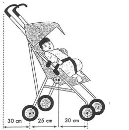
In order to lift the front wheels up and over a kerb on a footpath whilst moving forwards, the person pushing the pram must exert a downward force (F) on the handle. Calculate the minimum value of F.
