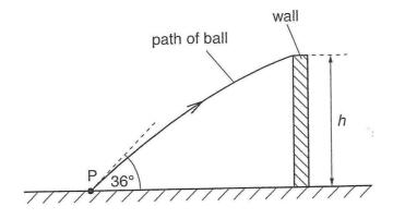
The initial velocity of the ball is 12.4 ms<sup>-1</sup> at an angle of  $36^{\circ}$  to the horizontal. The ball just passes over a wall of height *h*. The ball reaches the wall 0.17 seconds after it has been thrown.
