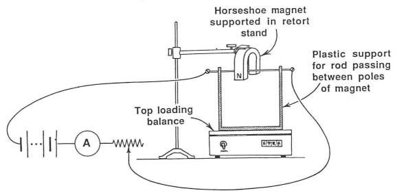
When the trial is ready to begin the "Tare" button on the electronic balance is pressed. This zeros the reading on the balance. The current was varied by adjusting the variable resistor (rheostat). Three trials were conducted for each value of the current used.
