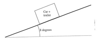
b) If the car is moving at a constant velocity, what is the resultant of these three forces?
