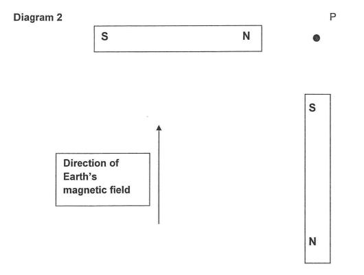
b) At point P on diagram 2, draw an arrow indicating the direction of the combined magnetic field of the bar magnets and Earth.
