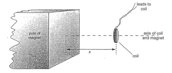
The coil has a cross-sectional area of 0.40 cm<sup>2</sup> and contains 150 turns of wire.
