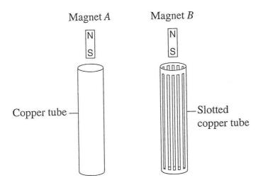
The magnets are dropped at the same time. Each magnet falls straight through its tube without touching the tube walls.
