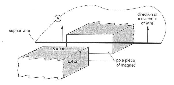
The magnetic field in the region between the poles is uniform and has strength of 89 mT.
